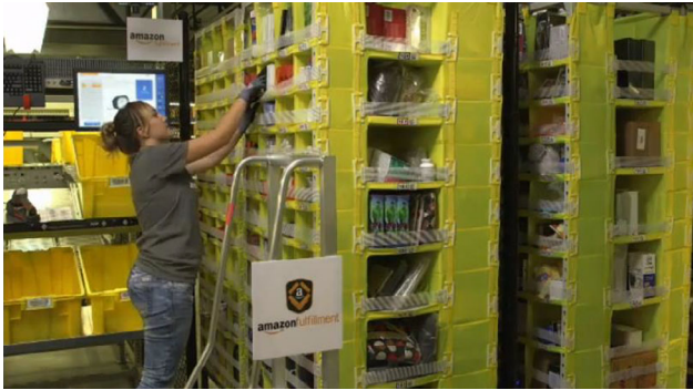
Figure 1 Order Picking in a Mobile-Rack Part-to-Picker System (Designboom, 2014) [Color figure can be viewed at wileyonlinelibrary.com ]
